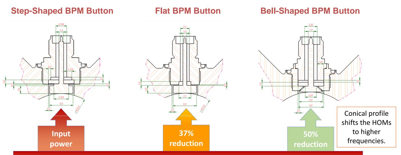
wakelosses calculated from electromagnetic (wakefield) simulations based on Alun Morgan and Guenther Rehm work and help
