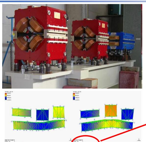
Figure 7: First vertical modal shape of girder at 116 Hz, girder on concrete stands
